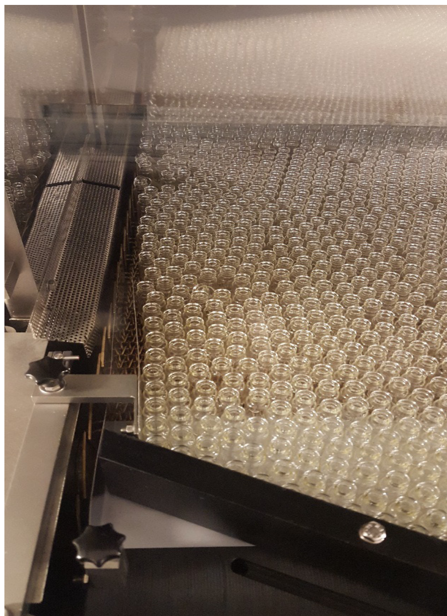
Figure 1 “En Masse” Movement of Glass on One of the First Trial Lines
